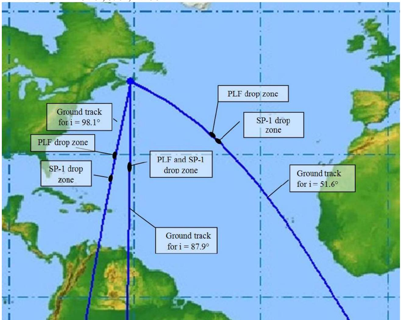
**Figure 2.1. Ground tracks and drop zones of Cyclone-4M ILV separated parts for SC injection into orbits inclined at 51.6°, 87.9°, and 98.1°**
